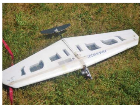
This close-up of Rod Christie's plane shows the unique cutouts that his daughter designed for him. They lighten the plane and, just maybe, entice her to fly.
