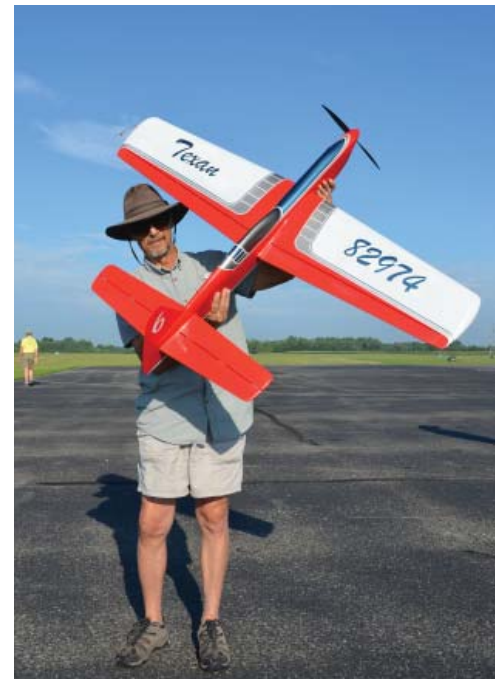
John Hill displays his original-design Texan that was based on a Crossfire wing. John's models are always beautiful and lightweight. This one is powered by a cast-case Jett 61, and it sports an Oliver pipe.
