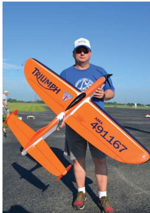
James Mills reprised his departed friend, Allen Brickhaus' design, the Triumph, as a tribute. The model is powered by a Cobra 3520-12 motor and a Zippy 4S 4,000 mAh battery pack.
