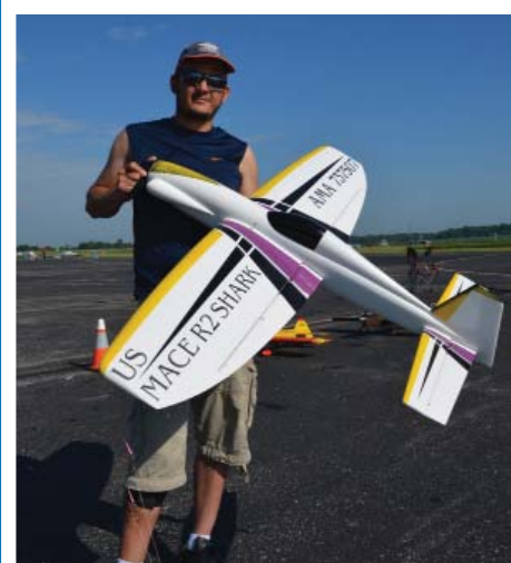
Josias Delgado is flying his Shark in Open this year. The electric model is powered by a RimFire 32 and a Thunder Power 5S 2,700 pack.
