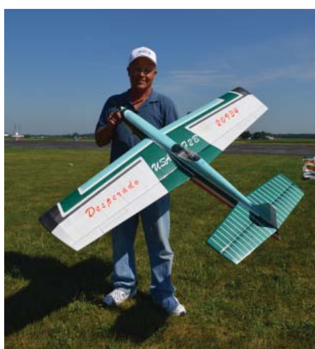
Dave Tribble has been refining his Desperado design for several years, and it appears to be a very competitive design. Dave prefers a Rojett 76 engine and a Smith/Werwage pipe.
