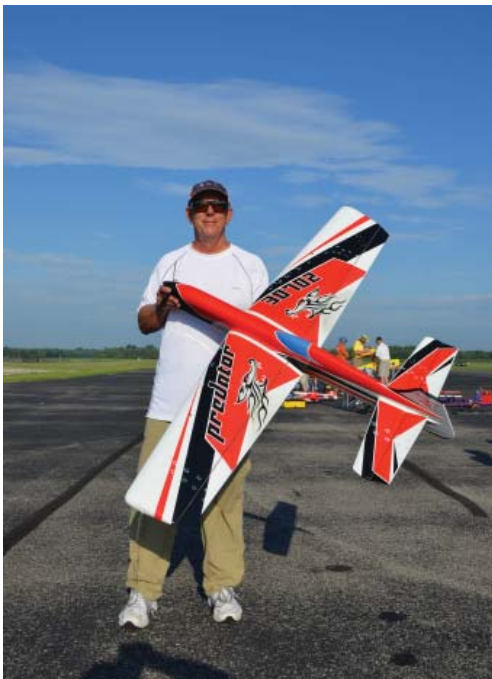
Here's our defending National Champion, Paul Walker, with his original-design Predator. Paul's aircraft is powered by a Plettenburg 1522 motor and uses a Thunder Power 6S 2,700 mAh battery pack.
